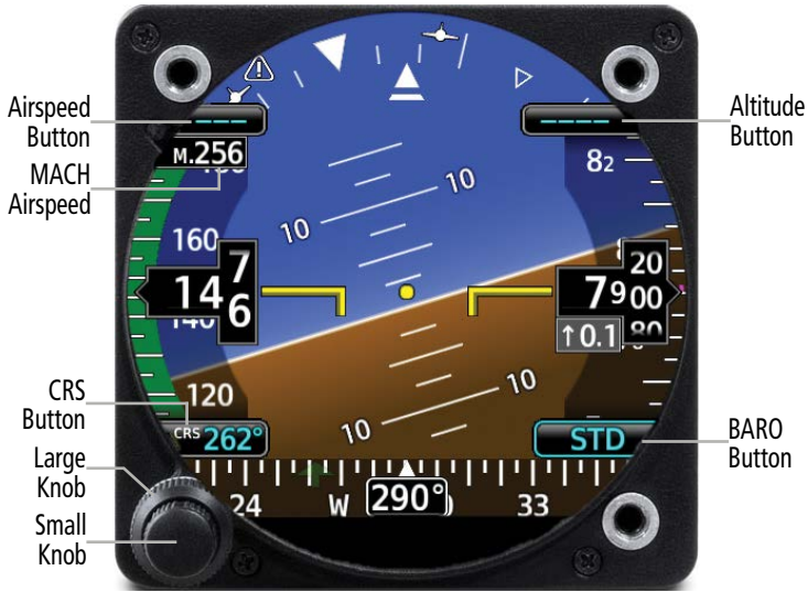
GI 275 Controls - Aircraft Symbol Change - MACH
