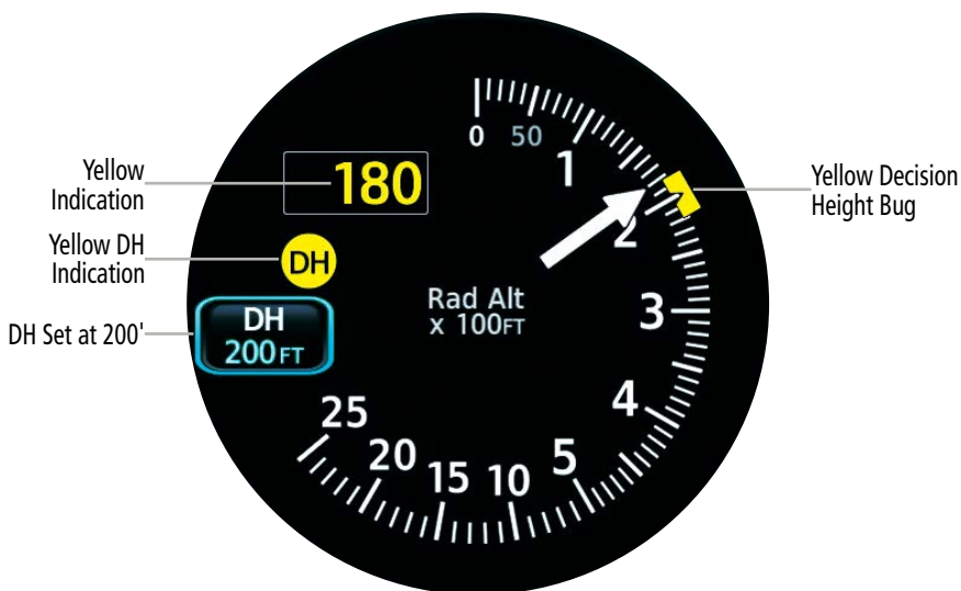
Airborne Indications - Below Decision Height - Fixed Wing
