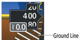
Altimeter - Ground Line
