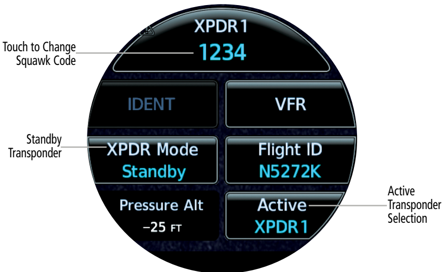
ADI - Transponder Control Display - Change Squawk Code
