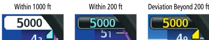
Altitude Alerting Visual Annunciations
